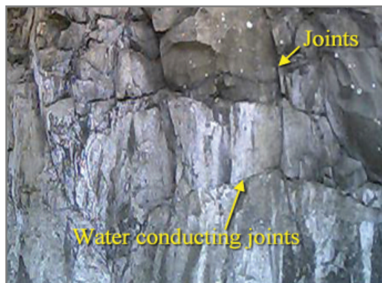
Typical Groundwater Pathways due to Intersecting Joints in Basaltic Formations – Trombay
