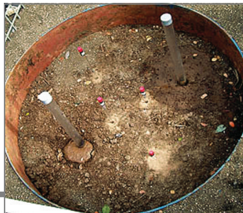
Lysimeter experiments include Time Domain Reflectometer (TDR) along with pore solution samplers
